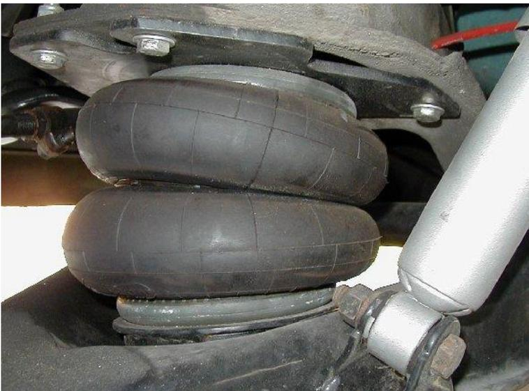
5. Bolt the lower bracket to the air spring using a 3/8" x 3/4" bolt, lock washer and flat washer.
