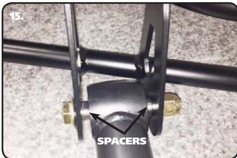
15. The StrongArms are a direct replacement of the factory trailing arms and will bolt to the new tubular cross member using two 5/8" x 4 1/2" Bolts, 4 Flat Washers, & 2 Nylok nuts. Insert the R Joint Spacers into each side of the R Joint. These bushings are Delrin and do NOT need lubricating.
