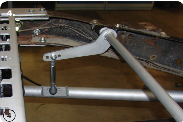
**4.** Attach the Posilinks in the **CENTER** hole of the MuscleBar and the StrongArm using a 3/8" SAE Flatwasher on each side of the arm on the MuscleBar and each side of the bracket on the StrongArm. Install 10mm Nylock nut on each posilink and tighten down.
