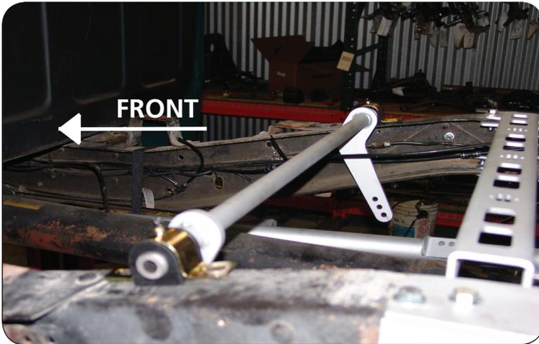
**Note:** This picture illustrates where the MuscleBar is positioned on the frame for drilling the holes. The Swaybar is located in front of the "C"-Notches against the bed support. The arms on the MuscleBar drop down and point to the rear of the truck. On 67-72 Trucks the bed support will aid you in positioning the mounts. On 63-66 the rear tab of the swab bar mount is 5 1/2" from the front of the "C"-Notch (Diagram #3).
