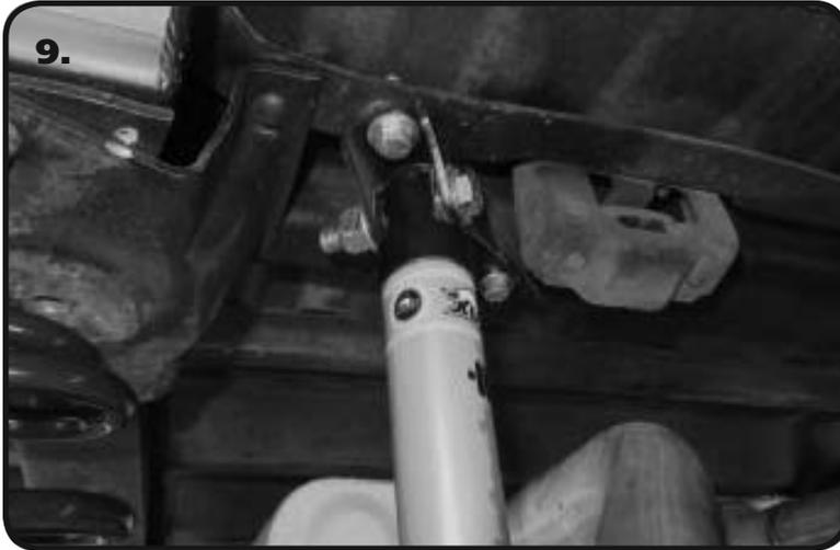
9. The Shock is mounted in the Upper Mount with the BODY UP. It is held in place with a 1/2"-20 x 2 3/4" Hex Bolt & 1/2"-20 Nylok with a 1/2" Flat Washer on each side of the bracket.
