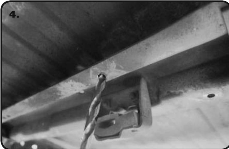
4. Drill the 4 rivet holes out to 7/16".
