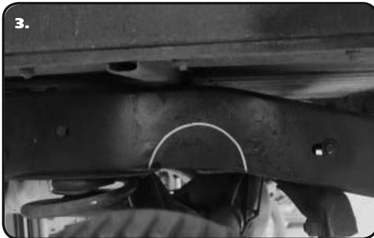
3. Diagram "3" shows the frame rail marked before cutting. The bottom of the frame will also need marked for cutting.
