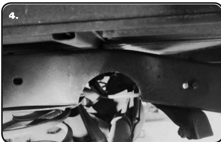
4. Diagram "4" shows the side and bottom of the frame after it has been cut.
