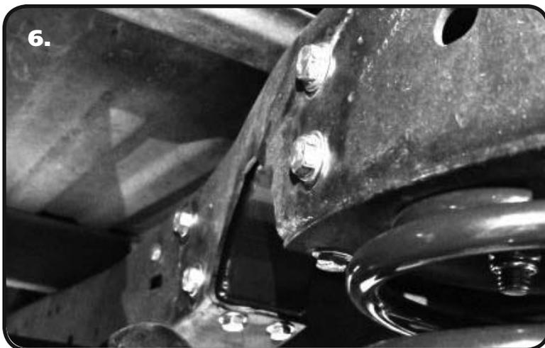
6. Install a 7/16" Flat Washer on (4) 7/16"-14 x 1 1/4" Hex Bolts. Insert them through the holes in the frame side. Install a 7/16" Flat Washer and 7/16"-14 Nylok. Install a 3/8" Flat Washer on (4) 3/8"-16 x 1 1/4" Hex Bolts, insert them in the bottom holes and install a 3/8" Flat Washer and 3/8"-16 Nylok Nut on the threads sticking through. Tighten all hardware and repeat on other side.
