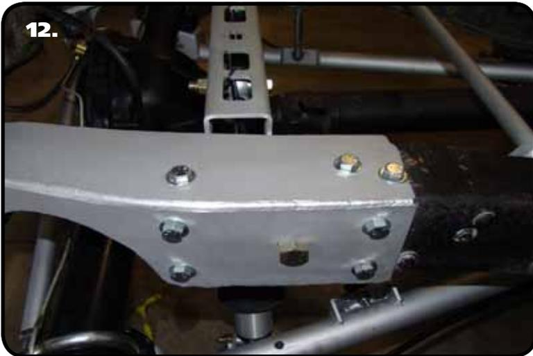
12. Once both "C" Notches are in place bolt in the upper shock bridge. The new upper shock bridge uses the (3) holes in the top of the "C" Notch. The bridge is offset to the rear of the truck, it goes from "C" Notch to "C" notch under neath the top lip of the frame sandwiching the frame between it and the "C" Notch. It is bolted in place using (6) 7/16" x 1 1/4 bolts, Nylok nuts and flat washers.
