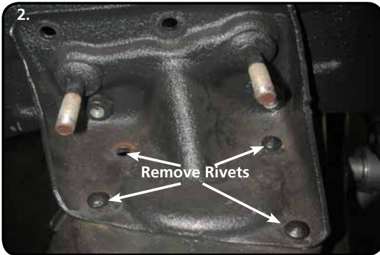
2. The factory upper control arm mount will need to be removed from the frame. There are 4 bolts attaching it to the frame rail with 4 rivets attaching it to the crossmember. There are several methods that can be used to remove the rivets from the crossmember. One way is to cut a "+" in the head of the rivet and chisel the 4 pieces of the head off the rivet, then knock the rivet out of the frame with a hammer and punch.
