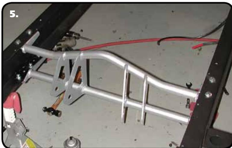
5. Install the new cross member with the trailing arm flanges towards the rear. The cross member is bolted to the bottom side of the frame rails using 10 - 7/16" x 1" bolts, 10 - 7/16" Nylok nuts and 20 - 7/16" flat washers. It may be necessary to enlarge some of the holes with a 7/16" bit.
