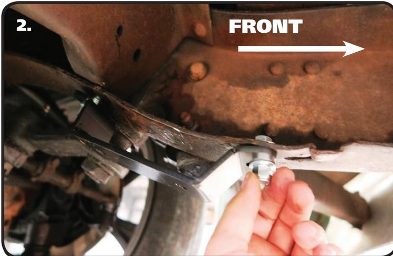
2. The MuscleBar Mount attaches to the frame using the holes from the OEM mount. The end of the frame bracket with the angled bends goes forward. Attach the bracket using a 3/8"-16 x 1 1/4" bolt, 3/8"-16 Nylok nut and a 3/8" Flat Washer on top and bottom. The same hardware setup is used in each hole. Repeat on the other side and tighten hardware.
