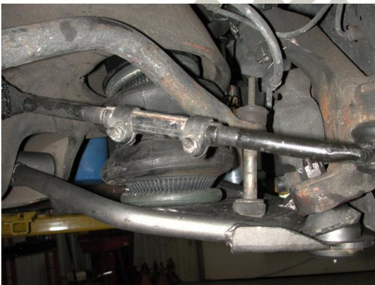
3. Slide the ball joint boot over the stud, then push the stud up through the spindle. Secure w/ the new castle nut and cotter pin supplied.
