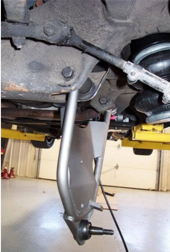
1. After removing the factory lower control arm, clean the bushing mounting surfaces on the frame and lubricate with the lithium grease supplied.
