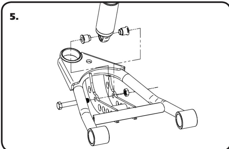
5. Raise the lower arm up to the Shockwave and bolt them together using the 1/2" x 3 1/4" bolt and Nylok supplied w/ the lower arms. An aluminum spacer will be on each side of the bearing. Torque to 75 ftbs.
