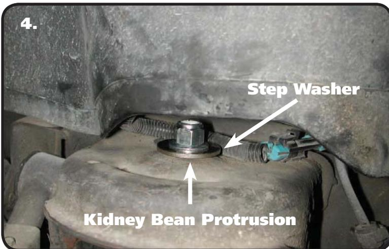
4. Raise the Shockwave up to the coil spring mount with the carriage bolt sticking through the factory shock hole. The hole in the frame is larger than the bolt, so a step washer is supplied. This should be installed on top of the frame, followed by a 1/2" Nylok nut.
