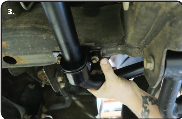
3. Slide the SwayBar into position on the truck. The SwayBar Arms will be above the steering linkage. Install Bushing Straps Over the Poly SwayBar Bushing and bolt them in place using the OEM hardware. Do not tighten the hardware until the PosiLinks are hooked up to the MuscleBar.
