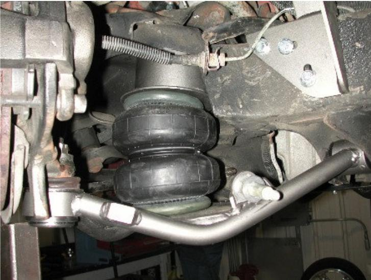
4. Attach to the air spring & shock to the lower arm using the hardware supplied w/ those kits.
