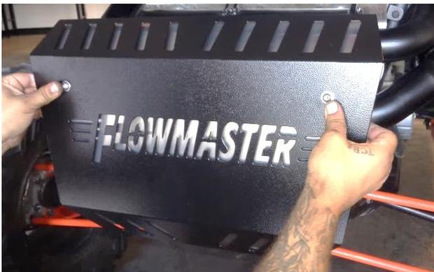
15. Grasp the aligned heat shield, backer and hardware and hang the assembly on the muffler's 2 top mount holes. Then install a flat washer (7) and lock washer (9), and hand-start a nut (10), on each screw.
