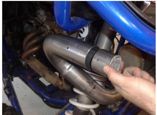
3. Remove the spark arrestor screen.
