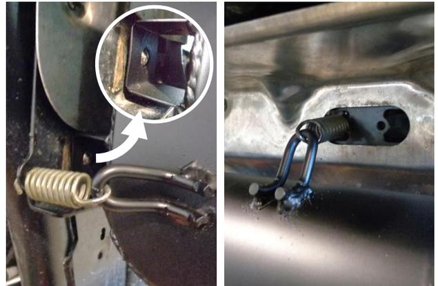
11. At the lower left corner of the muffer, center the alignment hole over the bump on the forward heat shield. Then use a spring puller to connect the 2 muffer mount springs to the new muffer.
