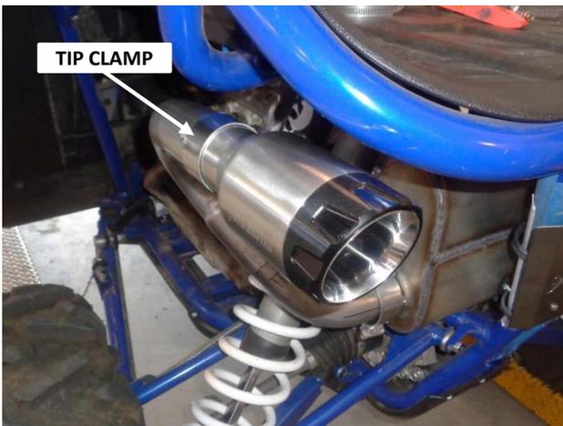
1. Loosen the exhaust pipe tip clamp and remove the tip.
