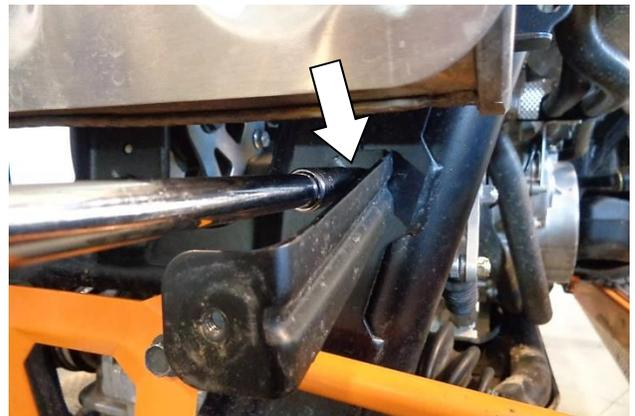
5. Remove the 2 lower heat shield brackets (one below each end of the muffler).
