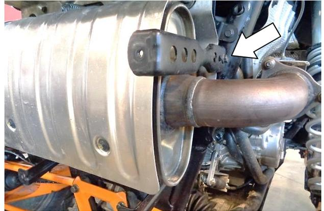
4. Remove the 2 upper heat shield brackets (one on each side of the muffler).
