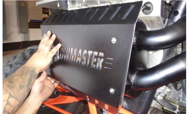
16. At each bottom hole, hold a spacer (8) in between the heat shield and backer. Install a screw (6) with flat washer (7) through the stacked parts. Then install a flat washer (7), lock washer (9), and nut (10) on each screw.
