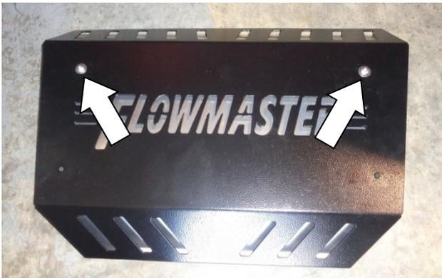
14. Place the heat shield (5) over the spacers and place flat washers (7) over the top 2 holes. Align the backer, spacer and the shield holes, and insert screws (6) in them.
