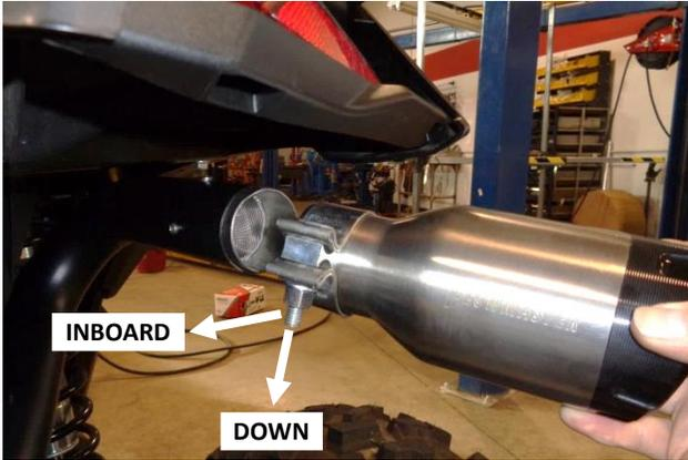
19. Note also that each clamp bolt should be on the inboard side of the tip, with its nut pointing down. Install each tip on its exhaust pipe.
