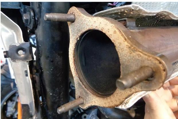
9. Inspect the exhaust flange gasket for serviceability. Replace if required.
