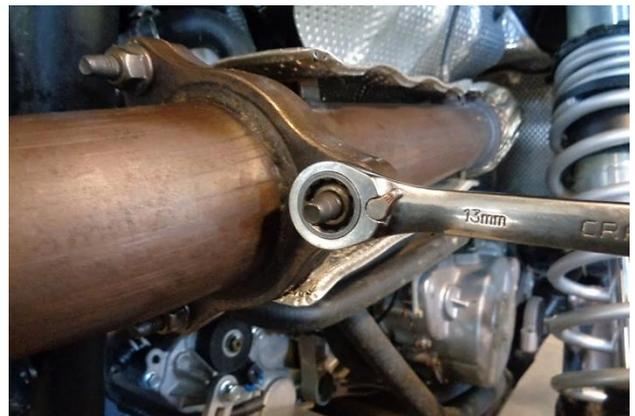
6. To prevent seizing of the flange nuts during removal, apply penetrating oil or anti-seize compound to the exposed stud threads. Then remove the 3 flange nuts.
