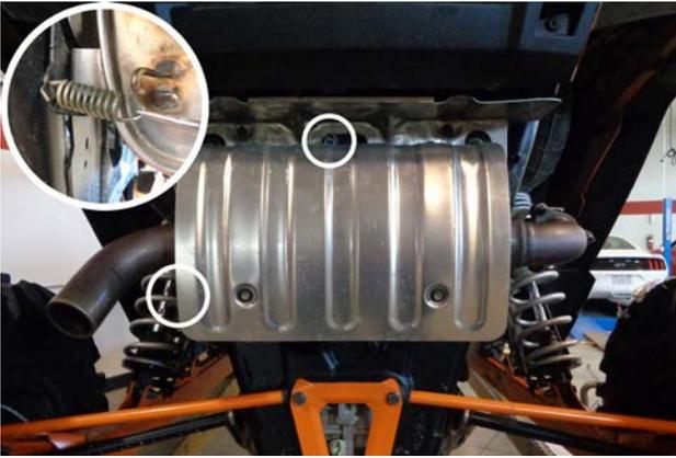
6. Use a spring puller to release 2 muffer mount springs.
