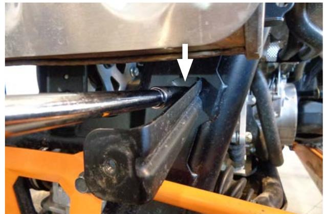
4. Remove 2 lower heat shield brackets below each end of muffler.
