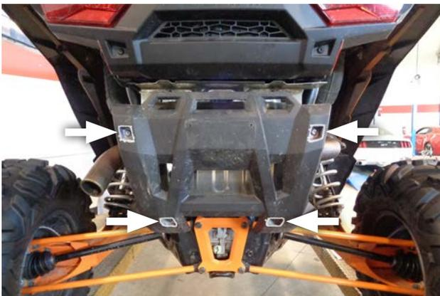
2. Remove 4 heat shield bolts and heat shield.
