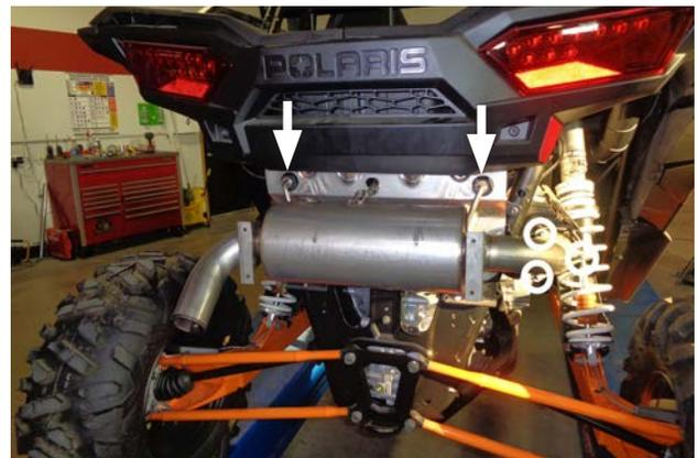
11. Install muffer by pushing 2 hanger pins into rubber mounts and matching 3 flange holes to studs at inlet connection.
