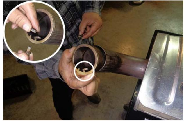
9. Remove bolt, washer and spark arrester from factory muffer outlet. Retain for later re-use.
