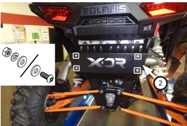
14. Install heatshield (2) over muffler using 4 screws (4), flat washers (5), split lock washers (6) and hex nuts (3). Tighten fastener assemblies completely.
