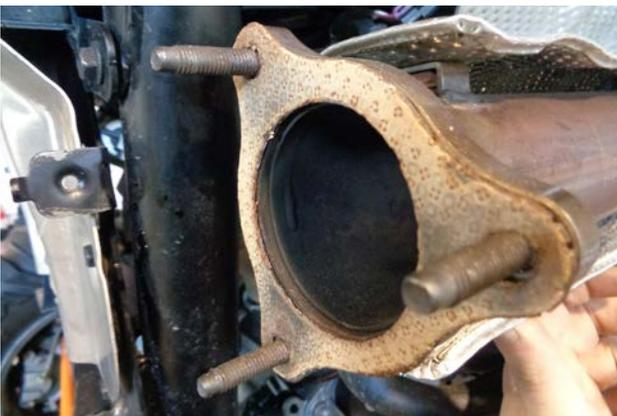
8. Inspect exhaust flange gasket for damage (cracking, etc.). Replace if required.
