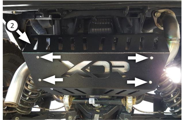
9. Install **heatshield (2)** to muffler using (4 ea.) **screws (4)** through **flat washers (5)**, mounting surfaces, **flat washers (5)**, **split lock washers (6)** and **hex nuts (3)** as demonstrated in cover drawing.
