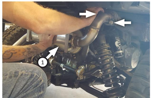
5. Place **muffler (1)** onto vehicle mount then partially thread bolts (x2) from previous step into inlet.
