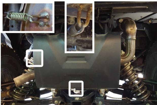
2. Dismount springs (x2) securing factory muffler to vehicle. Retain springs for later use.
