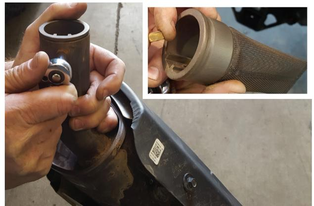
4. Remove nut, bolt and spark arrestor from factory muffler.
