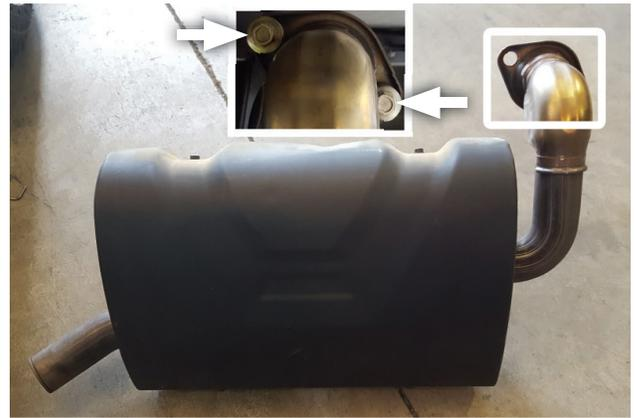
3. Remove bolts (x2) and muffler from vehicle. Retain bolts for next step.
