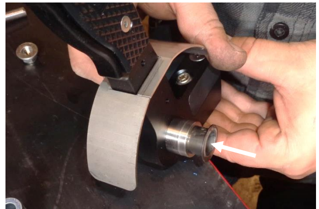
23. Press one stock plastic sleeve fully into each end of the steel pivot sleeve in the shifter assembly (1).
